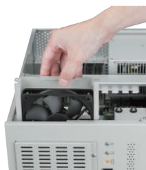
Easy-to-maintain cooling fan
